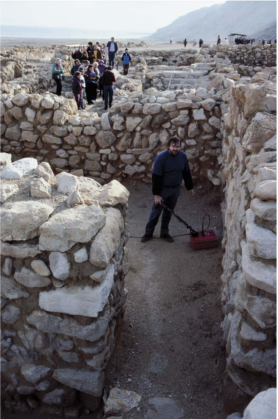
Operating the sensitive transducer for the ground radar system at the ruins of Qumran.
