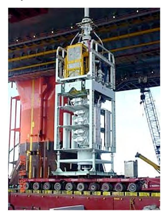
The BOP is like a big hollow assembly "Stack" with hydraulics attached to it that fire big sharp piece of steel called shear rams across the hollow that can snip the drill pipe clean off and seal the hollow shaft, like a dog nail clipper, but it stays closed.
